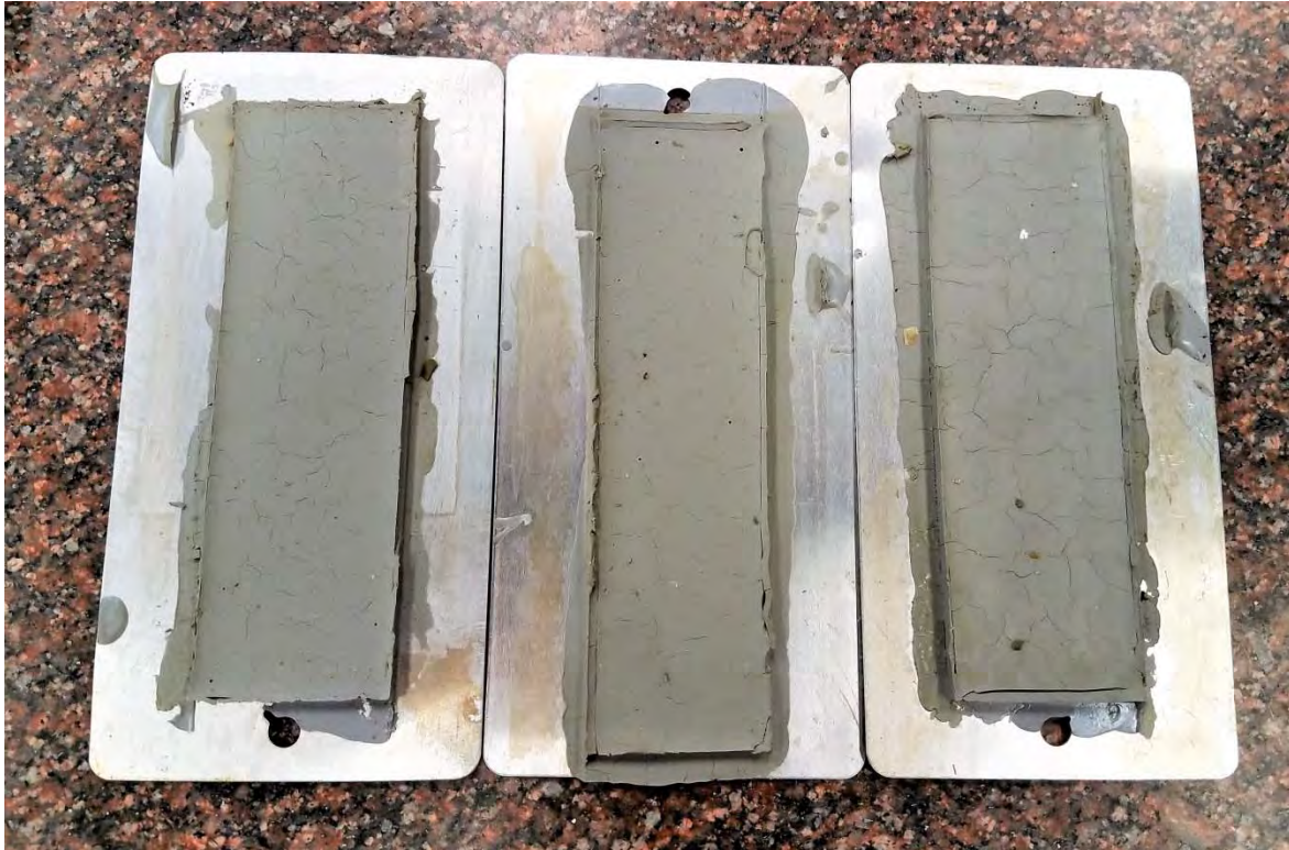
Photo 3 – Specimens following UV Exposure– ASTM C793
