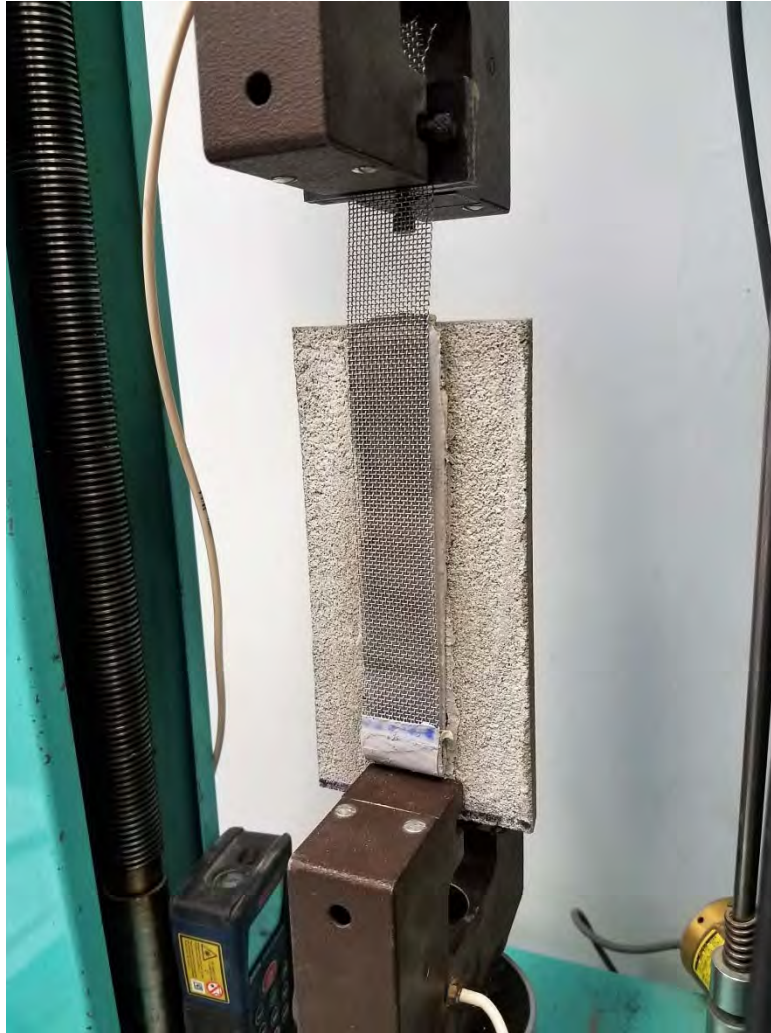
Photo 1 – Adhesion in Peel – ASTM C719
