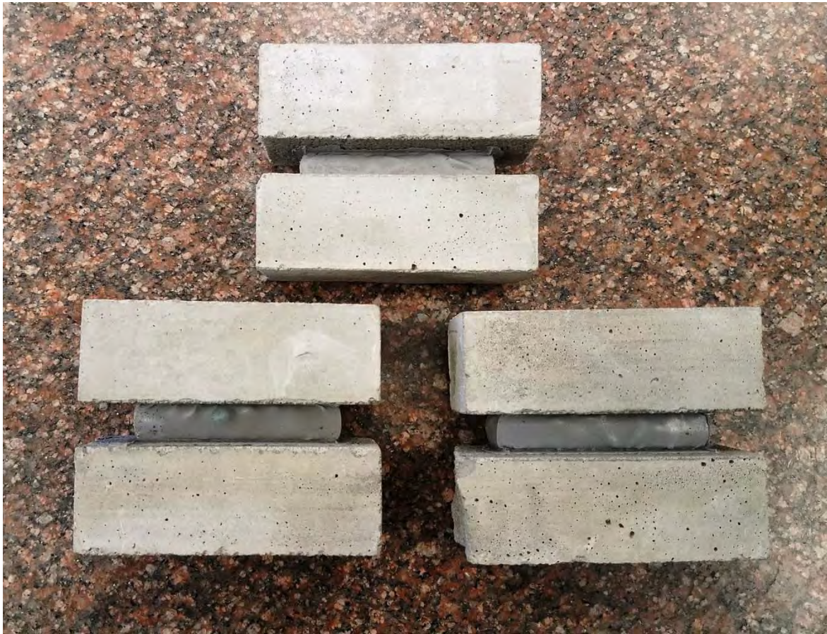
Photo 5 – Specimens after Extension/Compression Cycles – ASTM C719
