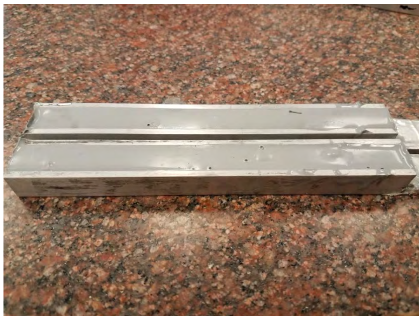
Photo 2 – Horizontal Displacement – ASTM C639
