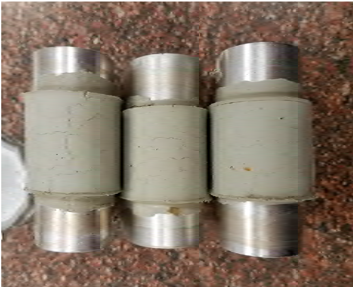
Photo 4 – Bend after Freezing – ASTM C793
